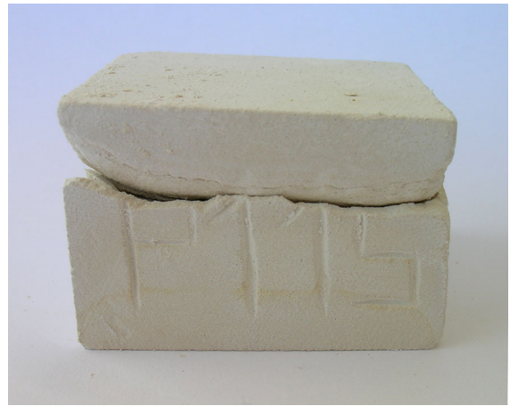
Fig. 5 Limestone specimen after incomplete saturation by partial immersion in a solution of sodium sulphate. Salt has accumulated at depth and led to spalling of a thick layer; this kind of damage is generally not observed in this stone on-site (Nunes C 2008, Methods for the artificial ageing of stone by salt crystallization for use in investigation of stone conservation treatments. M.Sc. dissertation, Instituto Superior Tecnico da Universidade Tecnica de Lisboa, unpublished)
