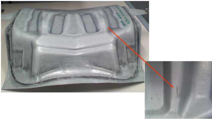
Figure 2: Sheet metal part formed with EHF process with multiple parallel cavities requiring substantial sheet metal stretching leading to splitting shown by the arrow.
