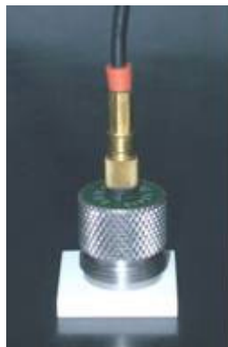
Figure 1. 5MHz longitudinal wave transducer, coupled to the pellet used in this study.
