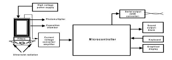
Figure 1. The Block Diagram of the Digital Fluorometer
