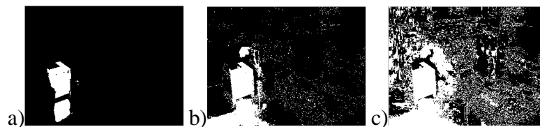
Figure 6. Effect of different binarization threshold level; a) level equal to 0.61; b) level equal to 0.45; c) level equal to 0.43.
