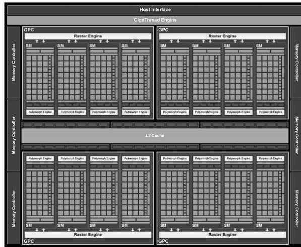
Fig. 3: Simplified GTX-480 GPU graphics processing architecture.
