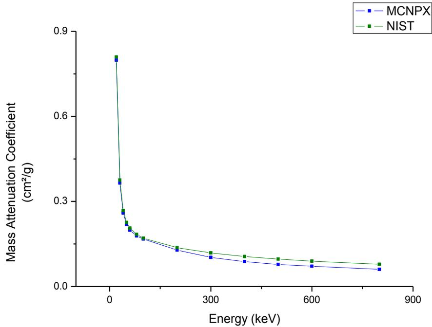
Figure 1: Comparison between NIST and MCNPX results.
