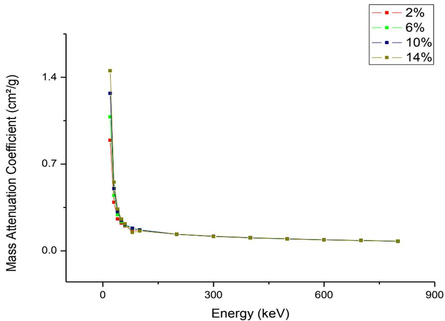
Figure 2: Mass attenuation coefficient in energy function, with variations in salinity. It is noted that the low energy region has a greater attenuation, presented in Fig. 3.
