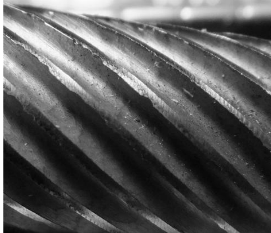
Figure 2.4: Chipping of the cutter teeth on the tool
