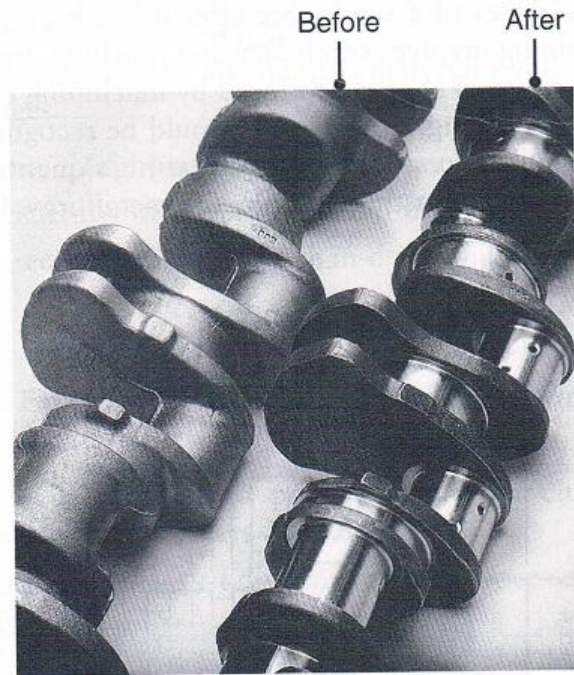
Figure 2.1: A forged crankshaft before and after machining the bearing surface
