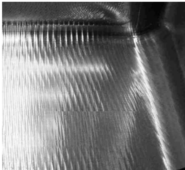
Figure 2.3: Poor surface finish of the product caused by the chatter of machining
