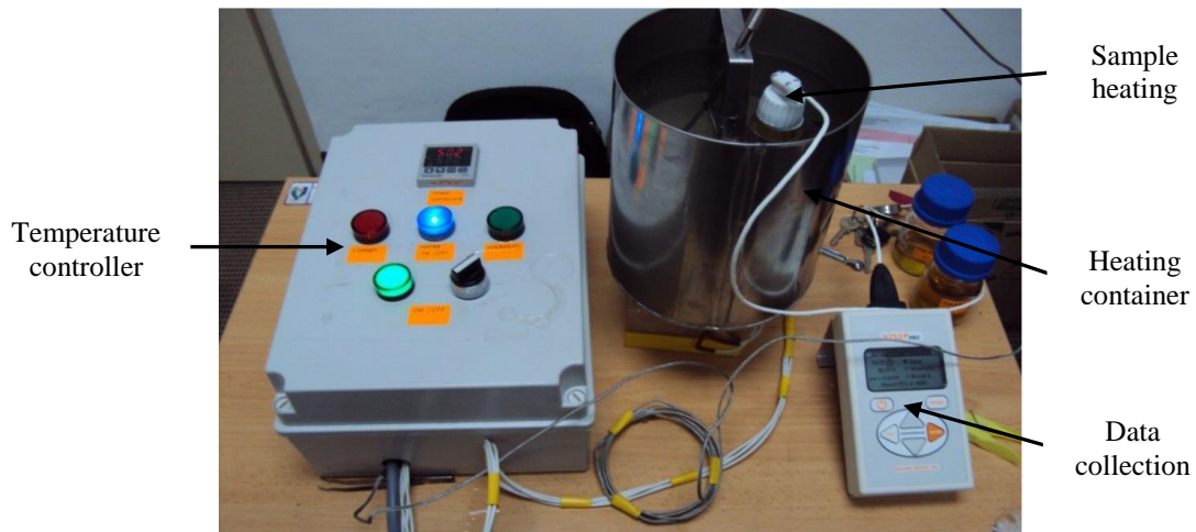
Figure 2. Water bath setup to test the fuel properties.
