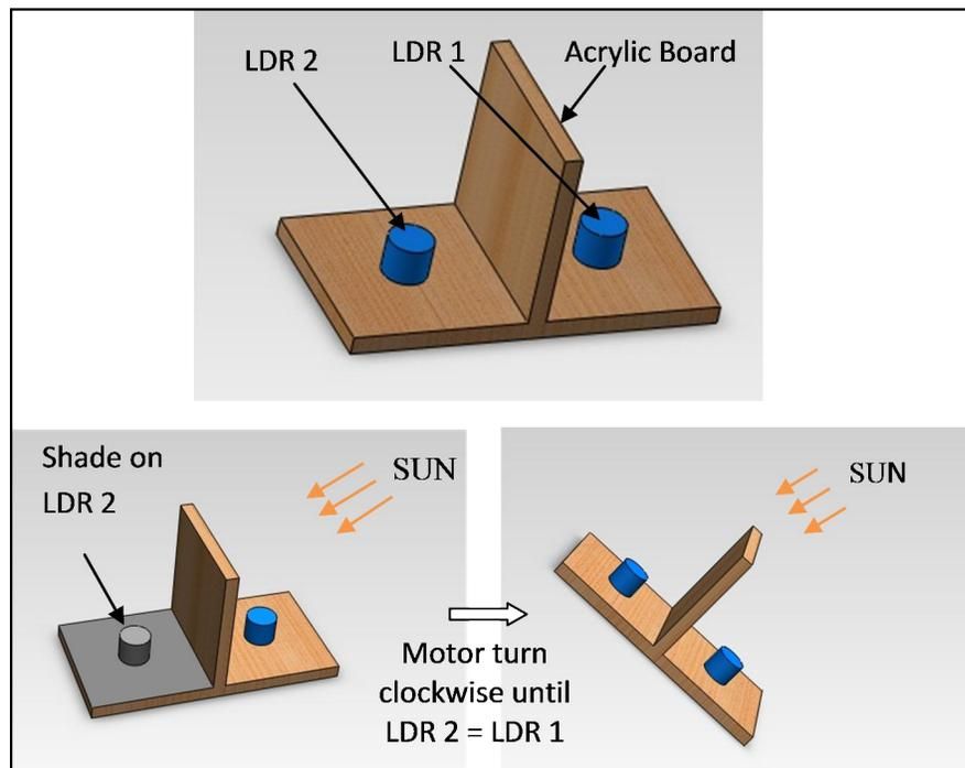
Figure 3. Tracking system working principle using LDR
