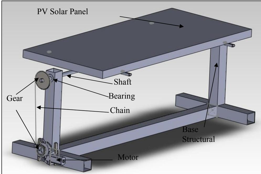
Figure 2. CAD drawing of Single-axis tracking PV
