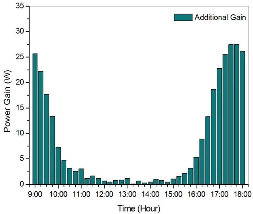
Figure 5. Additional power gain from single-axis tracking solar panel on a clear sky day
