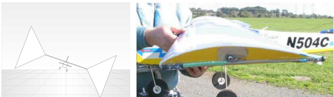
Figure 22: Wingtip thermopiles sensing rolling motion in reference to the horizon (Taylor et al., 2003).
