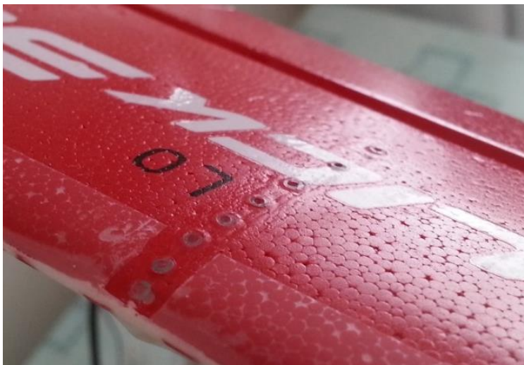
Figure 51: Pressure taps embedment on the suction side wing surface
