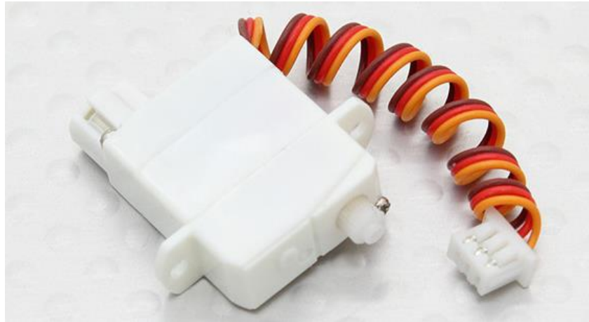
Figure 47: Micro digital servos.
