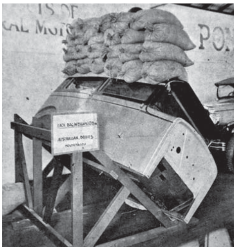
Fig. 7.13 1928 Adelaide Motor Show stand showing a Holden Motor Body builder's sedan body loaded with wheat bags.
