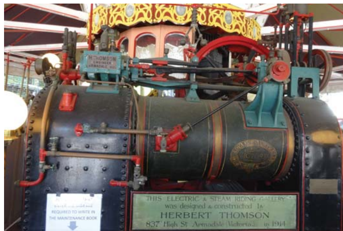
Fig. 2.25 & 2.26. Two versions of Thomson stationary steam engines. Left. A vertical unit at the National Steam centre Melbourne and above the 1914 carousel engine made for the St Kilda council and now in Canberra.
