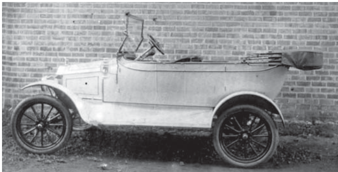
Fig. 6.29 1913 Ford T deluxe body built by Melbourne Motor Body Works for Tarrant.
