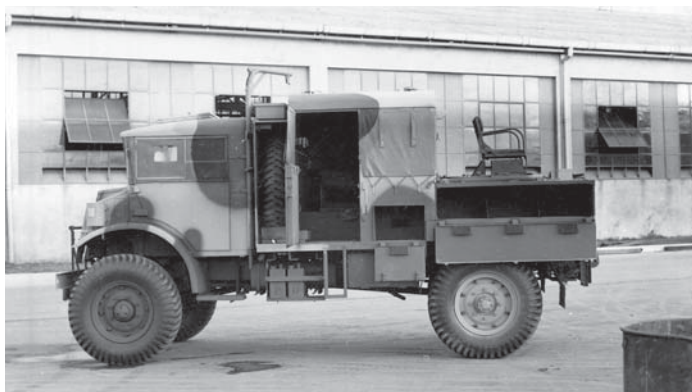
Fig. 8.23 Canadian War Office cab with GM-H modifications built for a Bofors Gun Tractor.
