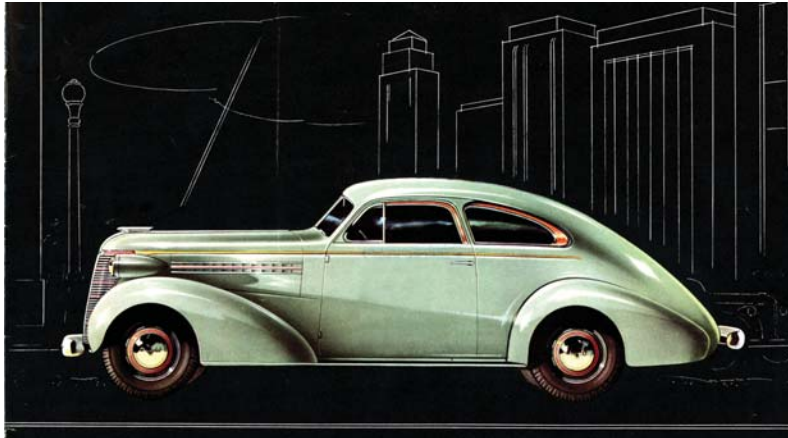
Fig. 7.47 The 1937/8 all-steel Holden All-Enclosed Coupé body on a 1938 Chevrolet chassis, Art Deco theme.
