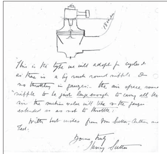
Fig. 2.45. Left and above. Sketch, drawing and notes by Henry Sutton describing his carburettor.
