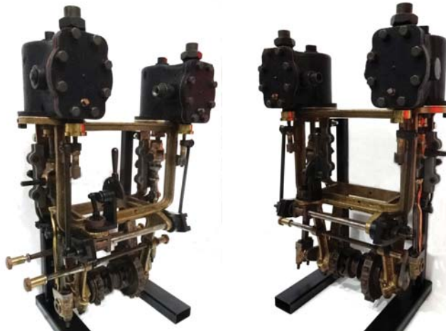
Fig. 2.19. Above. Two views of the Thomson steam engine as fitted to the 1902-5 vehicles.
