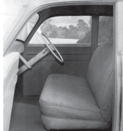
Figs. 8.54 & 8.55 1945 Dummy body at Woodville built, for trim development. GM-H Project 2000 folder
