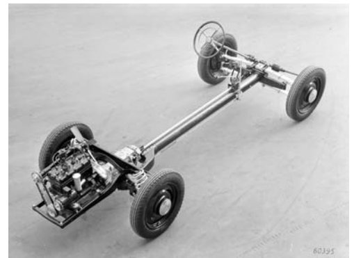
Fig. AII.11 Above. The Chamberlain 1938 proposed Australian car chassis compared to the Mercedes 130H chassis..
