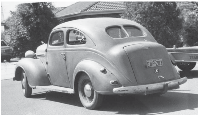
Fig. 7.51 T J Richards All-Enclosed coupé body on a 1937 Dodge chassis. N Darwin
