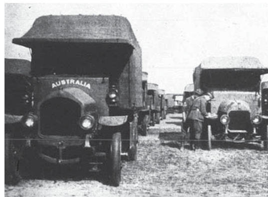
Fig. 4.2 Far Left. Ambulance design and construction was simple using timber and canvas.
