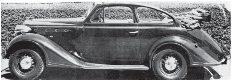
Fig. 7.49 Holden All-Enclosed Coupé Convertible roof body on a 1938 Vauxhall 25 chassis with a patented folding mechanism.
