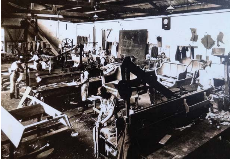
Fig. 3.17 Melbourne Motor Body works c1910. Chalk drawing of a roadster body propped on the wall. E Ford
