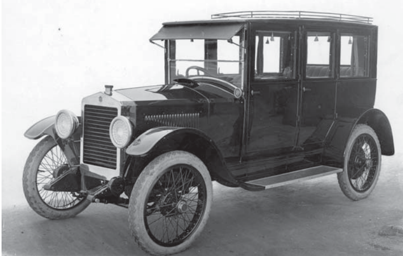
Fig. 6.24 1924 Essex chassis with HMBB's first sedan body. Somewhat dated in style with upright coach pillars. Holden - HMBB
