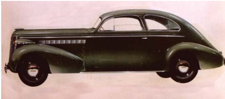
Fig. 7.48 The Holden 1937/38 All- Enclosed Coupé body on a long wheelbase 1938 Buick 8-cylinder chassis,
