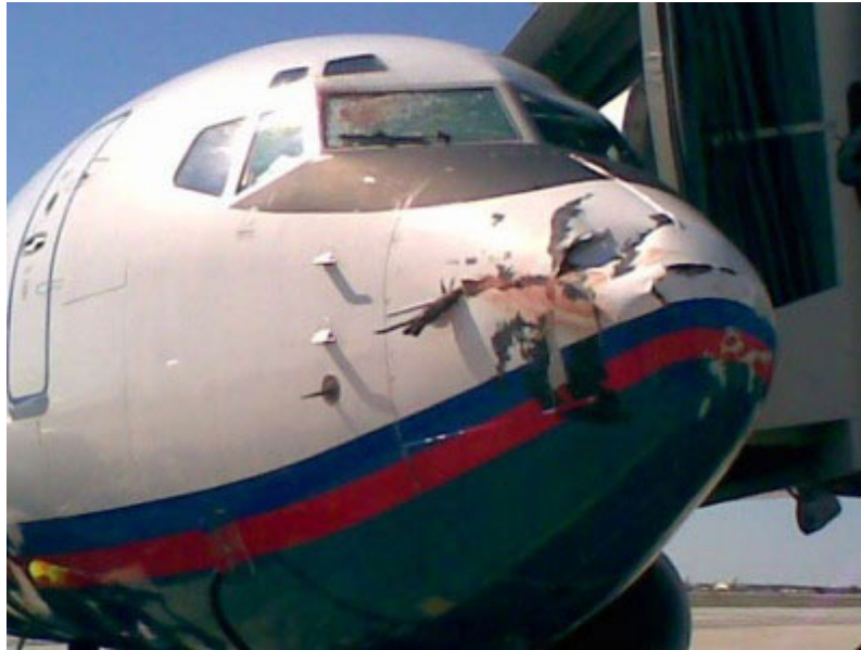
Figure 1.3 Damage to aircraft due to bird strike [20].
