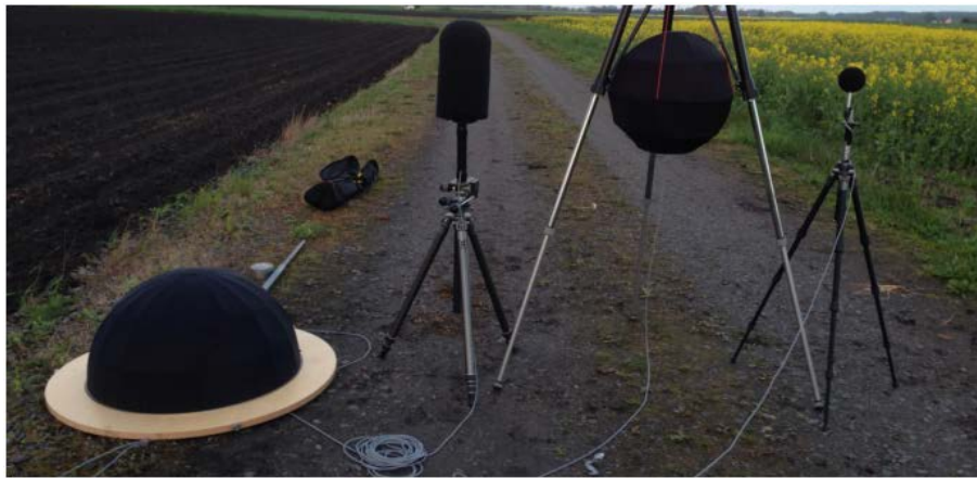
Figure 2.7 Experimental setup of Novak et al. [13] to compare the performance of 3 different secondary windscreens.
