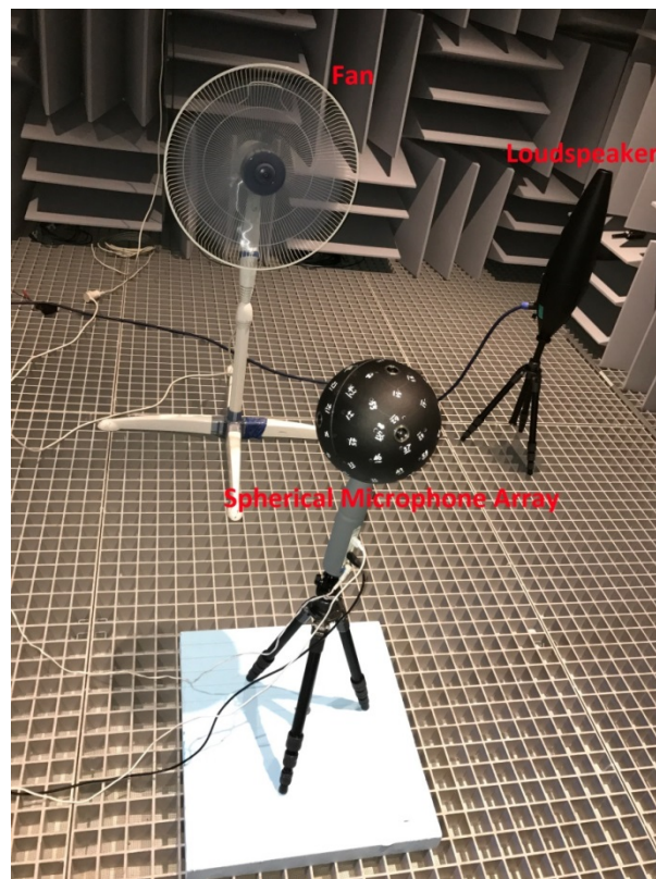
Figure 5.2 The experimental setup for wind noise measurement with a spherical microphone array in an anechoic chamber.
