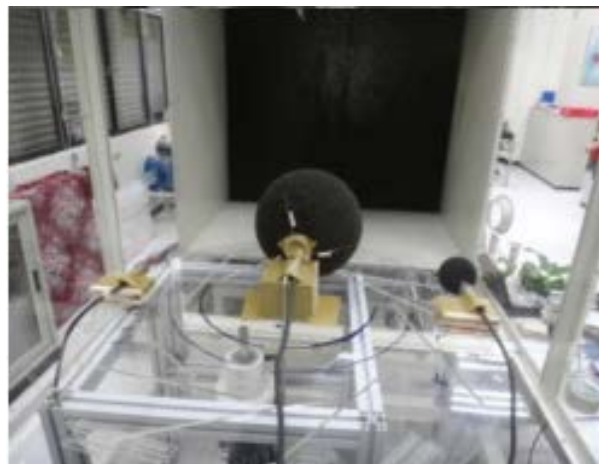
Figure 2.2 Experimental setup to measure wind noise inside the large (20 cm diameter) and small (7 cm diameter) porous microphone windscreen [47].
