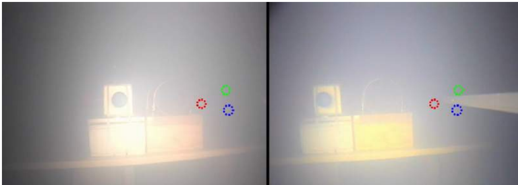
Fig. 6.15: Left and right camera images in experiment F. The dashed circles, which are not aligned with the target, represent the system's failure to recognize the target.
