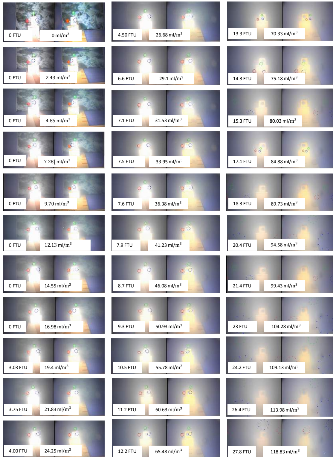
Fig. 6.8: Left and right camera images with the pose recognized by the pose estimation system at different turbidity levels and a distance of 600 mm between the ROV and 3D marker. The recognized pose is indicated by dotted circles in each photograph. The water turbidity measured by the turbidity sensor is shown in units of FTU, and the amount of added milk is given in units of milliliters per cubic meter.
