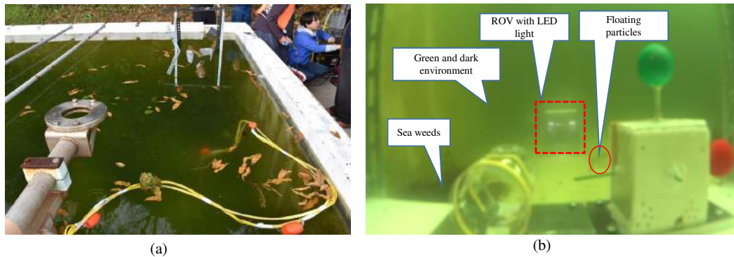
Fig. 5.12: (a) Turbid water in the pool, and (b) ROV and docking station.
