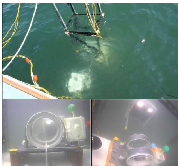
Fig. 6.17: Continuous iterative docking experiments in the sea. These photographs were taken by two underwater cameras installed in the docking station and from a pier.
