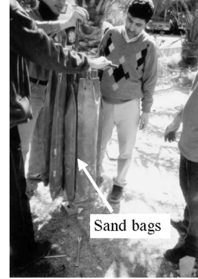
Photo 2. Swedish weight sounding at site of IIEES array 6.
