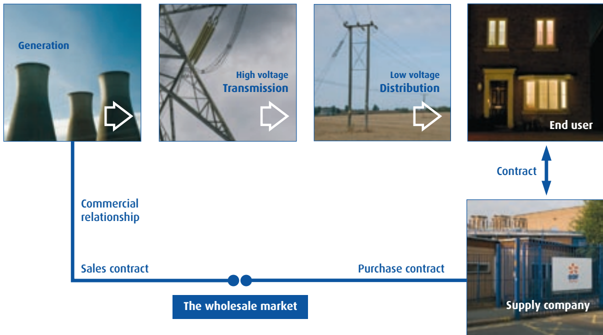
Figure 2 Technical flow of electricity
