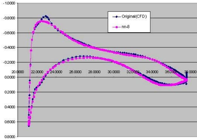
Figure 4: The plot of the output from the trained Neural network and the CFD calculations for one chord at one angle of attack and one mach number.
