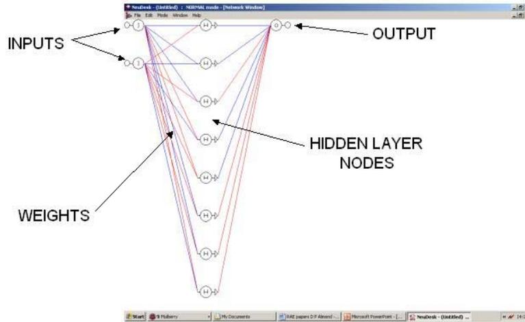
Figure 3: The layout of the nodes used in a trained neural network.
