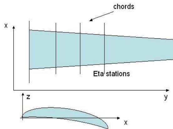
Figure 1: Diagram describing the layout of the wing and chords.
