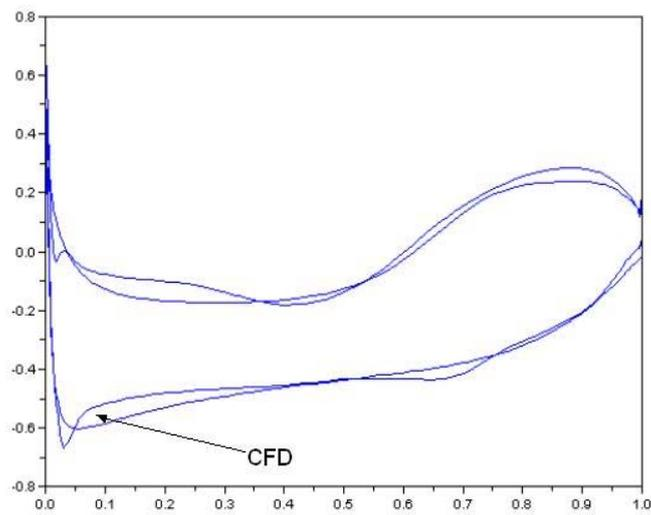
Figure 7: The output from a neural network trained using normalised arc length data at the wing tip.
