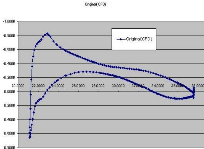
Figure 2: An example of the surface pressure coefficient data supplied by Airbus, calculated using a CFD package.
