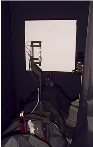
Figure 3.1: The picture on the left shows the Oriel lamp at Wallops in its bracket in front of the Spectralon plaque. The picture on the right shows James Yungel sliding the metal sheath over the Spectralon plaque. The circular 45° reflecting mirror can be seen in the center of the sheath.
