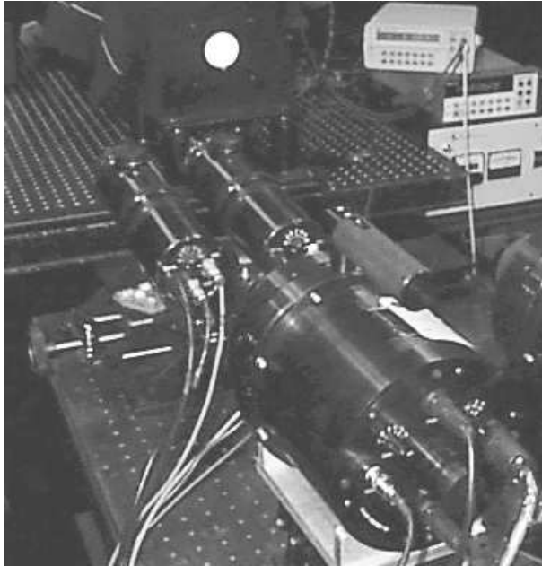
Figure 3.5: The two SLMs (center of the picture, in front of the SXR-II) on an optical table in the calibration cabin in Snug Harbor, Honolulu.
