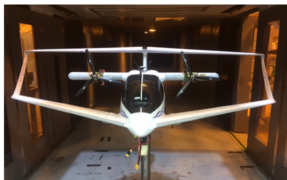
Fig. 1. Elytron 4S UAV in the US Army 7x10 subsonic wind tunnel at NASA Ames Research Center.
