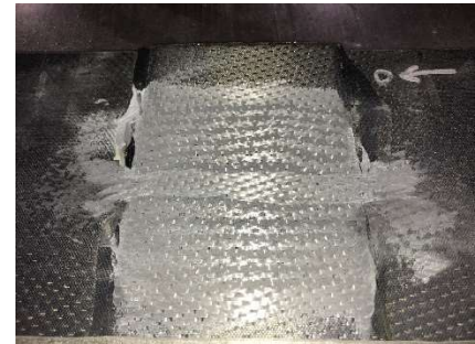
Figure 5. Tapered Scarfing on Test Panel Doubler
