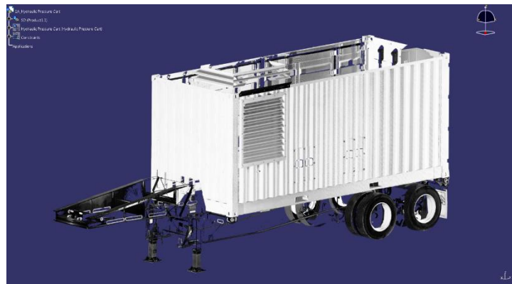
Figure 2. Point cloud of HPC scan that has been processed in RealWorks and imported into CATIA
