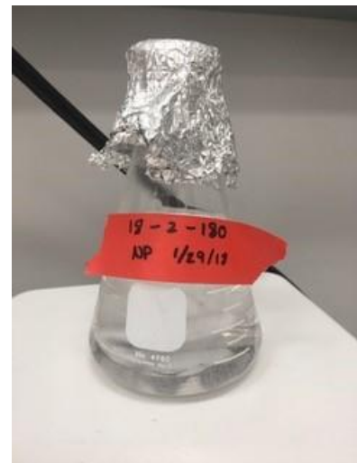
Image 1. A film solution clear of pullulan powder clumps after five hours of stirring.
