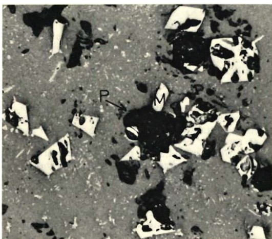
Fig. 11. Slag with 3.8 wt% lead: (M) magnetite, (P) metallic lead (magnification \times 400 ) [4].
