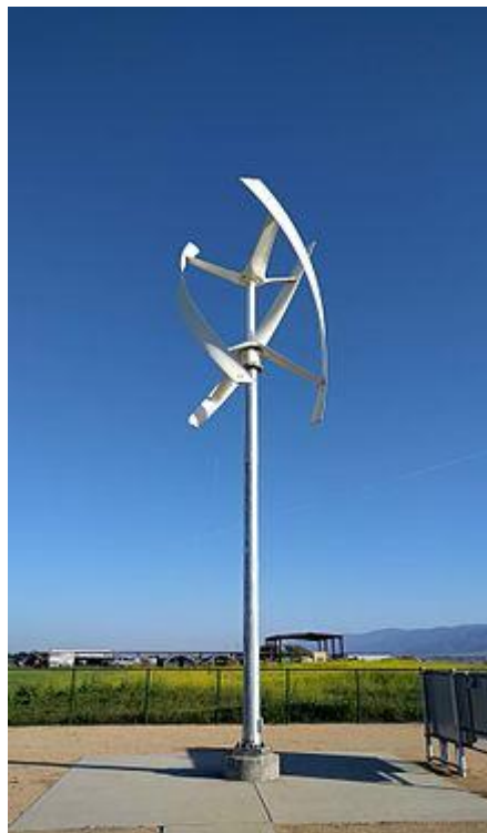
Figure 1.9 : A helical Darrius wind turbine.
