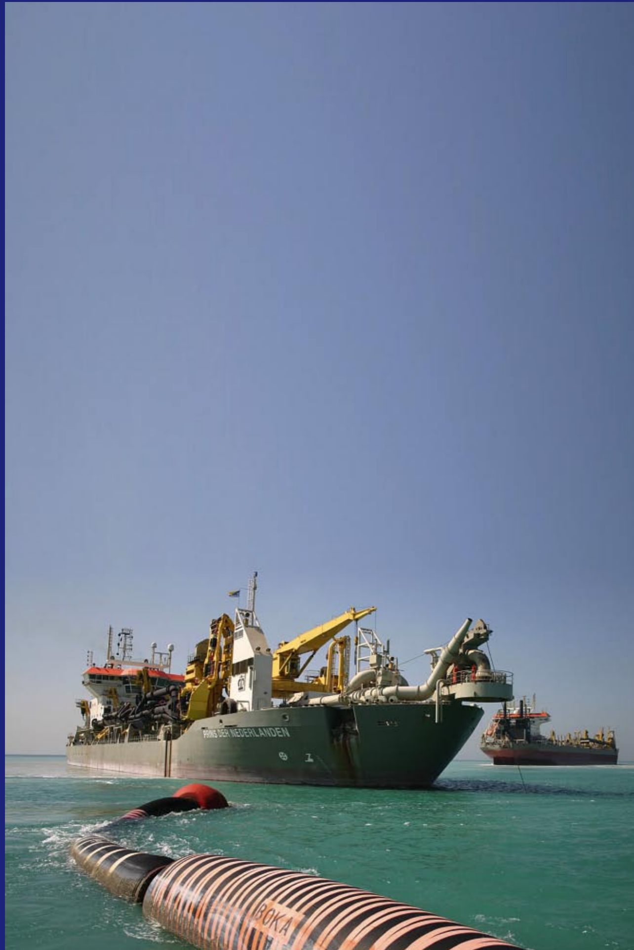
Figure 2.6.3 Trailing suction hopper dredger (Boskalis)
