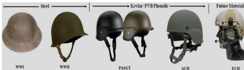
Figure 1.1 Historical perspective of U.S. Army helmet design and materials. PVB represents polyvinyl butyral. PASGT = Personal Armor System for Ground Troops. ACH = Advanced Combat Helmet. ECH = Enhanced Combat Helmet. Reproduced with permission from ref. 6. Copyright 2013 Elsevier.
