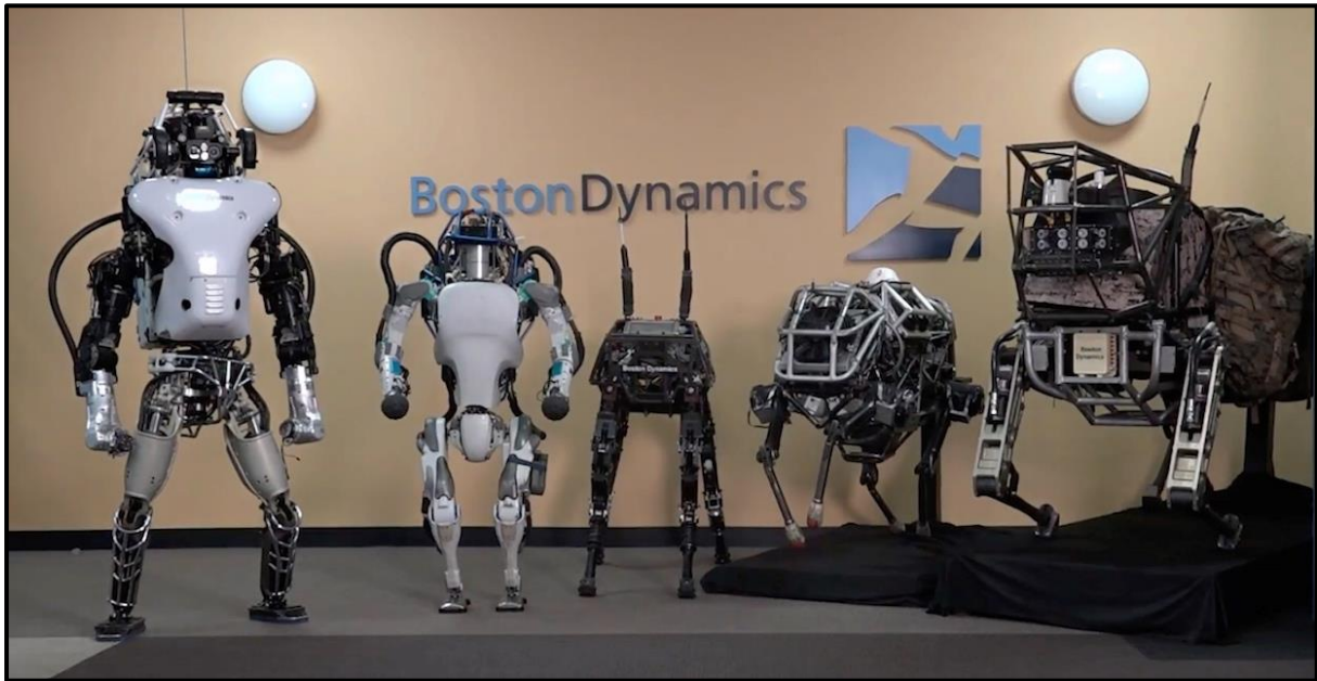
Figure 4.3: Atlas robot (2017) next to BigDog, WildCat, and AlphaDog
