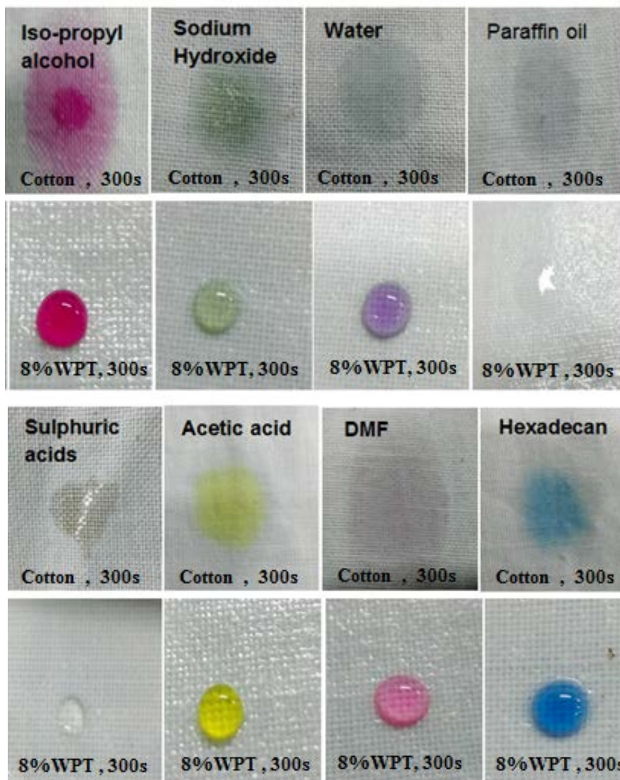
Figure 4-10: Chemical resistance after 300 second for coated fabric of 8% WPT and uncoated cotton fabrics.
