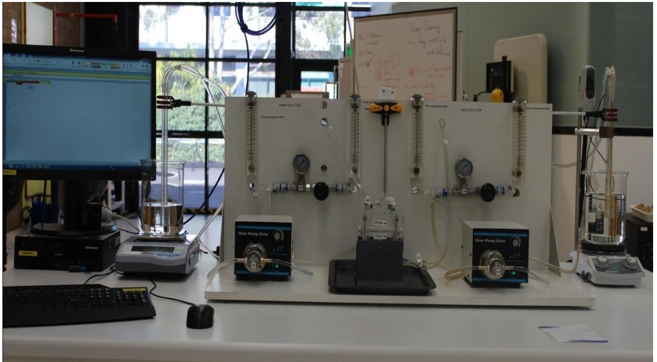
Figure 18: FO experimental setup used. Flat sheet FO module's membrane area is 33.54 \text{ cm}^2 .
