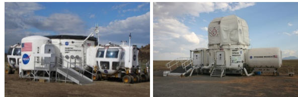
Fig. 2: GeoLab Glovebox integrated into the HDU: Pressurized Excursion Module for Lunar surface operations (left); HDU: Deep Space Habitat for cislunar operations (right).
