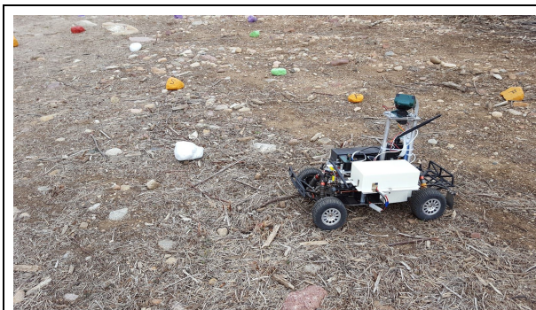
Figure 1. Modified COTS rover operated by human via low-latency teleoperations in search of exploration target.
