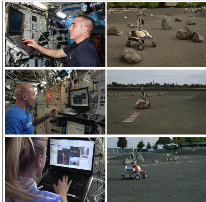
Figure 1. Surface telerobotics testing aboard the International Space Station during three crew sessions. Top: NASA astronaut Chris Cassidy surveys the NASA Ames “roverscape” site; Middle: ESA astronaut Luca Parmitano uses the K10 rover to deploy three “arms” of a simulated radio telescope array; Bottom: NASA astronaut Karen Nyberg remotely operates K10 to document the deployed radio telescope array.
