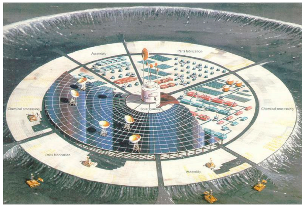
Figure 1 [1]: A 1980 self-replicating lunar factory concept that used autonomous robots in outwardly-growing sectors devoted to chemical processing, parts fabrication, and assembly.
