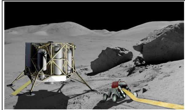
Figure 2. Surface teleoperation of a rover from the Deep Space Gateway is a key technology for astronaut-assisted deployment of a lunar farside polyimide antenna and the collection of geological samples. Image is courtesy of R. MacDowell and NASA GSFC.
