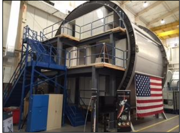
Figure 3. SLS-Derived Habitat Mockup: Layout is suitable for both a deep space laboratory and a Mars transit habitat configuration, (NASA, MSFC, Bldg. 4649).
