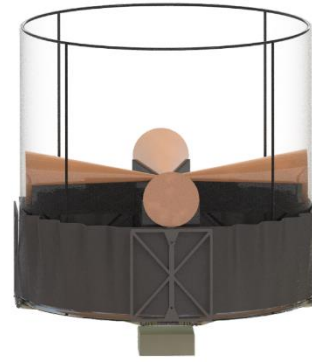
Figure 2: The antenna for the low frequency radio telescope is a pair of wideband orthogonal bicones surrounded by a cylindrical sunshade (shown transparent here for clarity). The antenna rests on a deployable ground plane and is connected to a temperature-stabilized backend consisting of a pilot-tone calibrated receiver and a high-resolution digital spectrometer.
