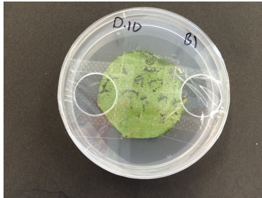
Figure 2-1: Bioassay chamber used in experiments to assess the virulence of EPF isolates against groups of DBM larvae.
