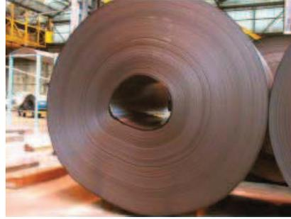
(b) Metal coil with racetrack bottom
