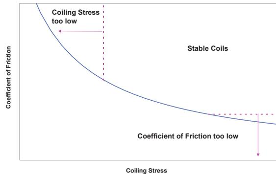
Figure 3: Critical tension-friction curve
