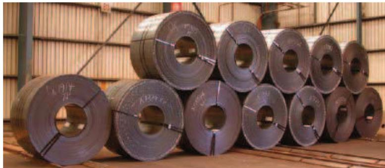
For BlueScope Steel, the long term objectives are: (1) the formulation of the governing equations for the stresses in a coil under self-weight, (2) the identification of analytical solutions and/or numerical schemes for the final coil shape after slumping, and (3) the formulation of exclusion rules-of-thumb which predict when a particular form of slump (oval or triangular, as illustrated in Figure 2 below) is likely to occur.
