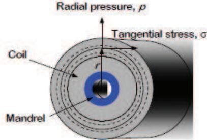
Figure 1: Basic Coil Geometry
