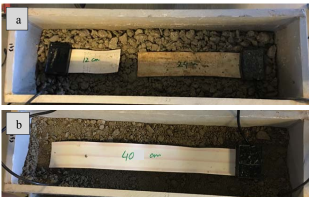
Figure 2. Placement of (a) 12 cm and 24 cm sensors after first layer compaction and (b) 40 cm sensor after compaction of second layer
