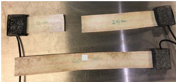
Figure 1. FRC sensors of three different lengths 12 cm, 24 cm, and 40 cm with black boxes to secure transition from coaxial cable to FRC
