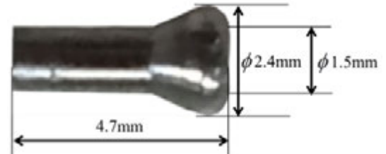
Fig. 4-10: The Endpoint Shape of the Thrust Wire
