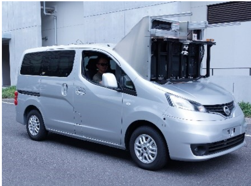
Figure 6.7: Exterior of the initial version of the experiment vehicle with the robotic camera hanging downwards from the linear motor mounted on top.
