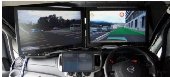
Figure 5.34: Interior of the cockpit with the two auto-stereoscopic displays. (Virtual windows)
