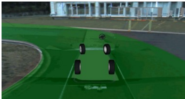
Figure 5.40: Close perspective birdview with a transparent representation of the own car and only the wheels and steering visible to help accurate maneuvering relative to the curb on the inside of the left turn. (Combined Geometric and Semantic enhancement)
