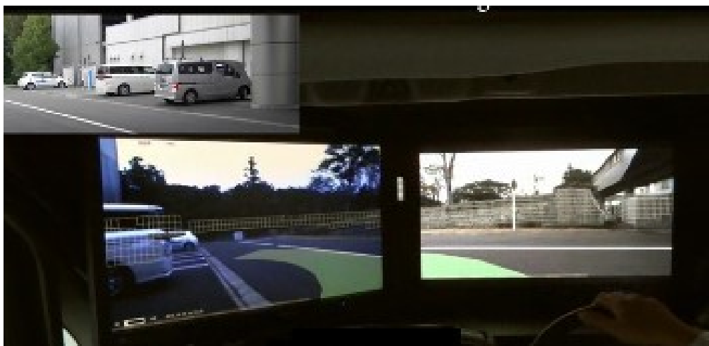
Figure 5.35: Life-size virtual rearview with a visualization of the expected trajectory. The image is left-right reversed in order to match the visual
