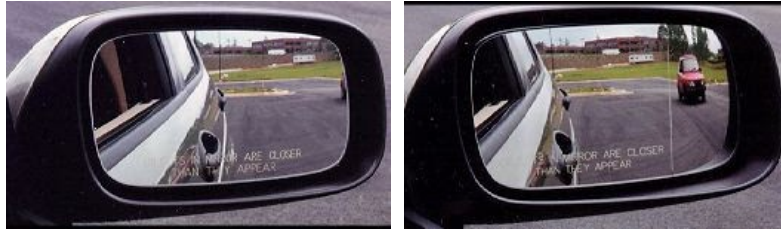
Figure 2.9: Conventional convex (left) and aspheric (right) door mirrors from a press photo by Saab. [19]
