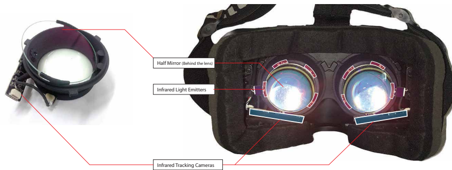
Figure 4.12: Eye tracking module used (PupilLabs + Oculus DK2).
