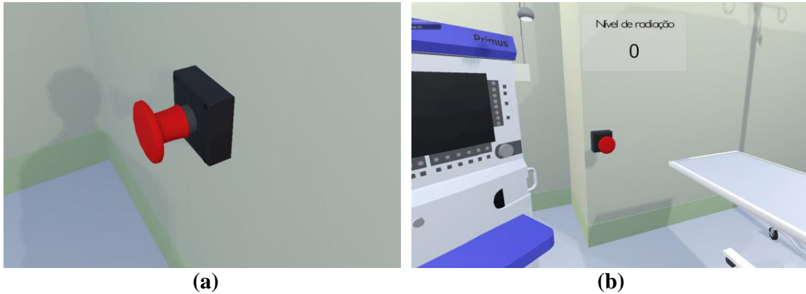
Figure 4: Emergency buttons; (a) in the bunker access; (b) in the bunker interior.
