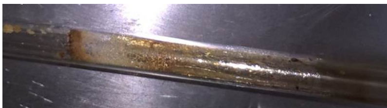
Figure C.1: Glassy deposits on the inner surface of the cold outlet of the reactor tube (quartz) after blank activity test at 400 °C with a feed of 3-3.5 mol% ethylene glycol, 27 bar H 2 , 550 ppm H 2 S, and 40 barg total pressure (balance N 2 ).
