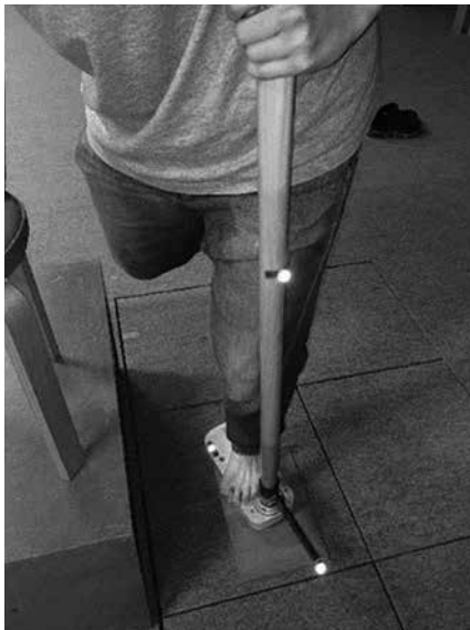
Figure 3. Subject applying weight vertically on the force platform.
