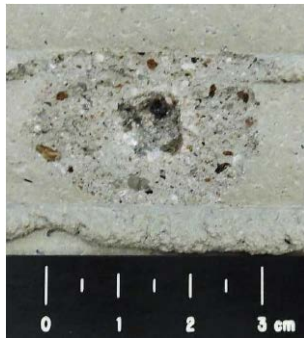
Martian simulant JSC Mars-1A, stucco mix, OPC, Navitas, and water
