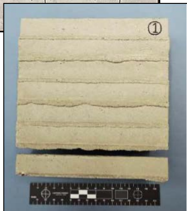
Sample delaminated during shipping to JSC on a boundary between prints made on different days
