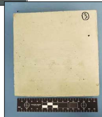
Lunar simulant JSC-1A, stucco mix, OPC, Navitas, and water
