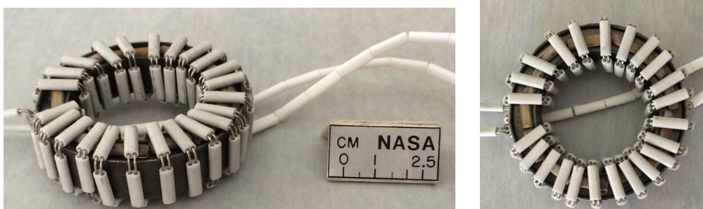
Figure 2.—Hiperco 50 test article equipped with excitation and sensing coils.
