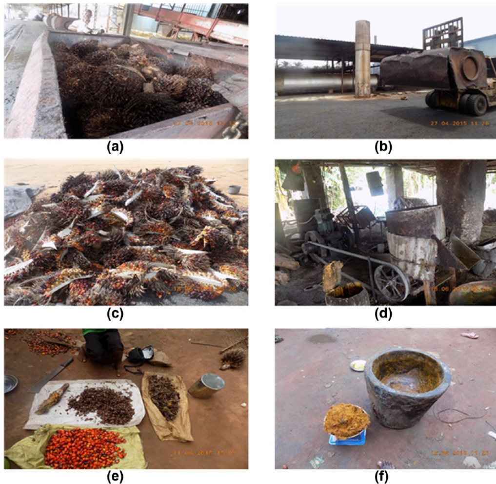
Figure 1. (a) sterilized FFB from industrial route; (b) part of the facilities of industrial route; (c) quartered FFB from small-scale route; (d) part of the facility of the small-scale route; (e) bunch stalk, empty fruit spikelet and fruits from traditional route; and (f) wooden mortar from traditional route use in fruit digestion.
