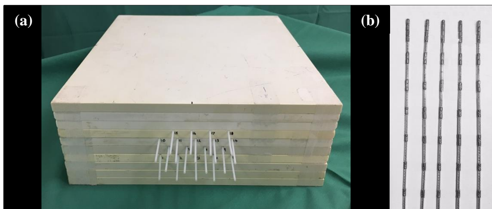
Figure 5.1. (a) The rectangular solid water phantom containing 18 plastic catheters and 3 fiducial markers positioned on the CT couch ready for the planning scan. (b) A sample of the radio-opaque dwell position markers with 10 mm spaced lead markers used during x-ray imaging.
