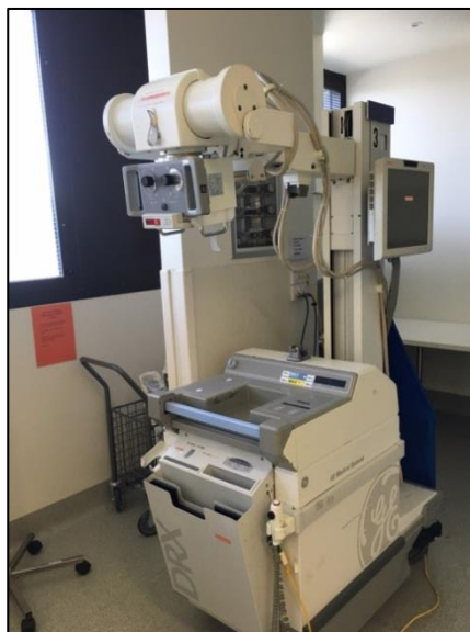
Figure 7.4. The mobile x-ray system GE AMX-4 model from Radiology department used initially for 2D pre-treatment image verification.
