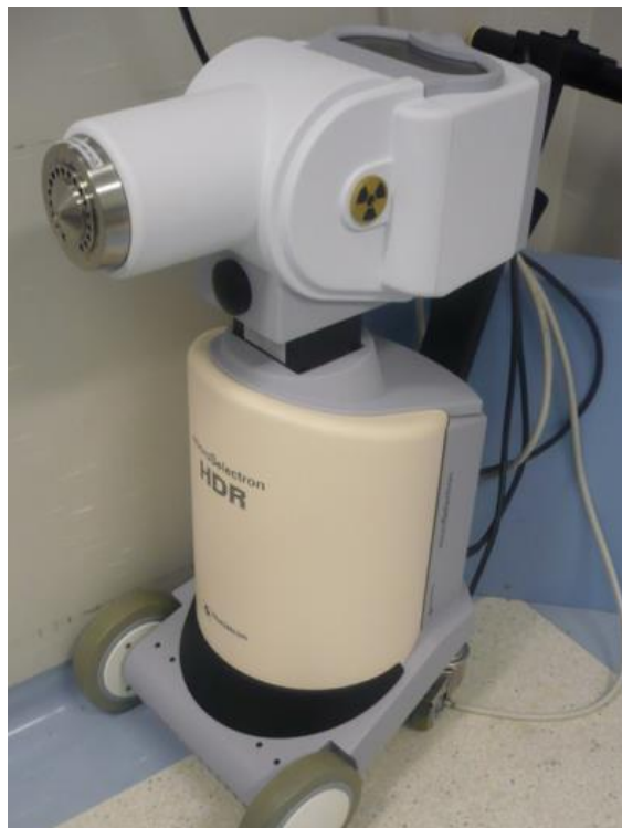
Figure 1.1. The microSelectron HDR brachytherapy robotic afterloader used in this work from Elekta ( Elekta, Stockholm, Sweden).
