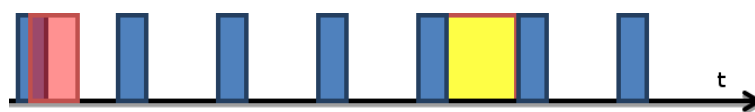
FIGURE 4.6: Wastage of Slots - Yellow box represented as SU transmission, Red box being PU transmission.
