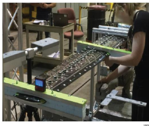
Figure 12. Photogrammetry testing of APV-3 wings.
