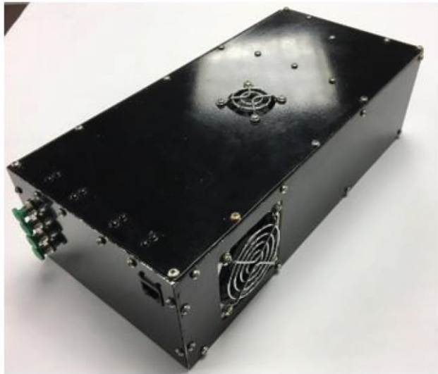
Figure 3. The compact fiber-optic strain sensing system.
