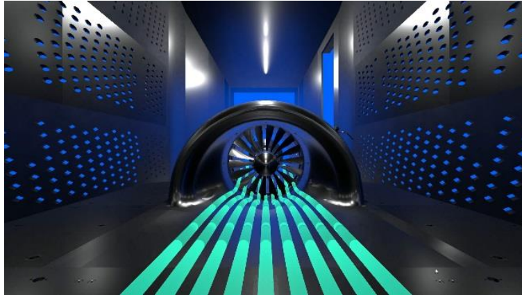
Fig. 1 Large-scale boundary layer ingesting propulsor experiment with simulated streamlines
