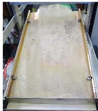
Figure 4: Copper tilt tray with uniform soil distribution. Heaters are mounted on the backside.
