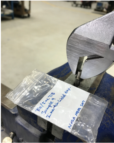
Figure 6. Sample being bend tested.
