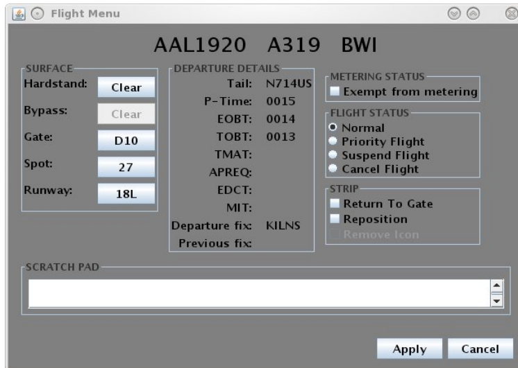
Figure 19 - The flight menu for flight intent contains entries for spot, runway, hardstand, and flagging for a priority flight.
